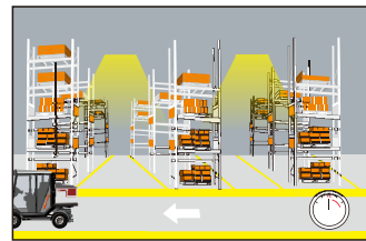
After hold time, the sensor dims the lamp at a low light level if no new motion trigger.
